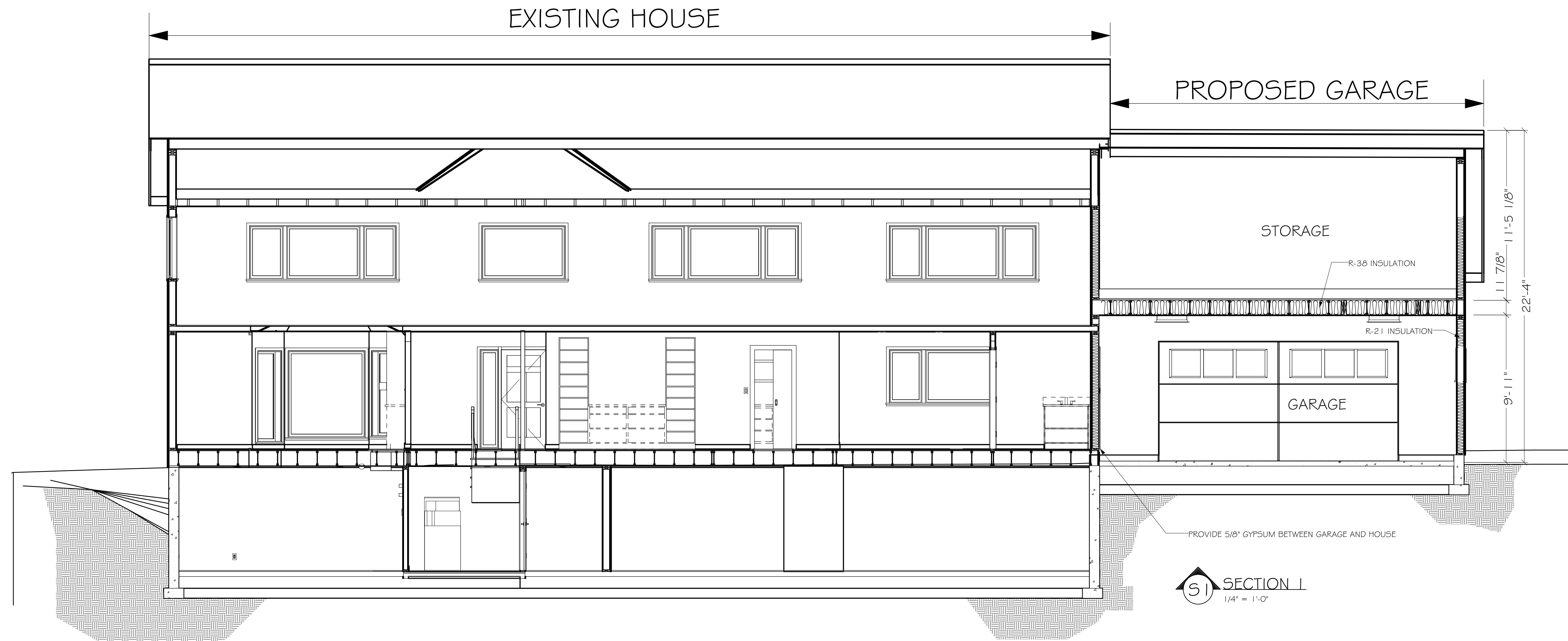
E3 REAR ELEVATION VIEW 1/4" = 1'-0"
